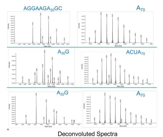
The poly(A) tail is digested into two main poly(A) populations based on the RNase specificity confirming the presence of the non-adenosine residues.
